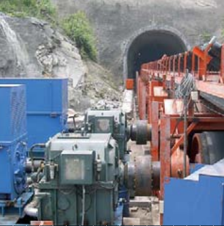
SINOHYDRO Xian Jia Ba Project, China. (31km, 5 flight conveyor system)
