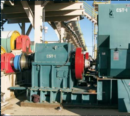
Thunder Basin Coal Mine, USA (3 x 2500K CSTs with flywheel and 2,500HP Baldor motor on skids)
