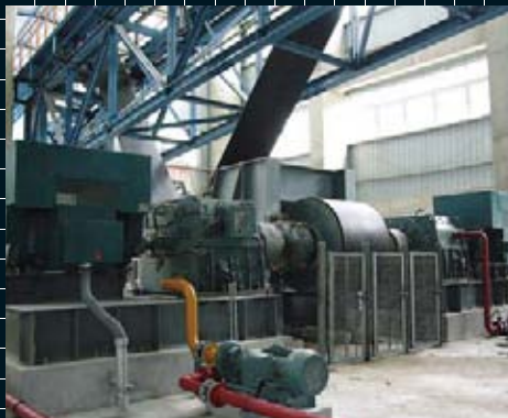
Dexing Copper Mine, China (6 x 1120K CSTs and Baldor motors)
