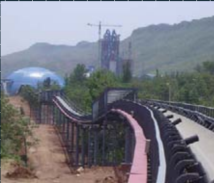
Yulong Cement Plant, China (8km conveyor with tripper drives)
